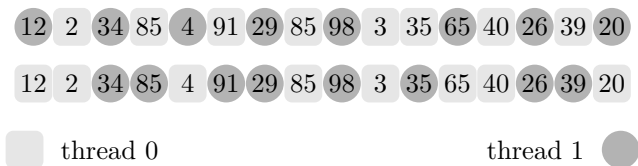
Figure 5: Two possible random number sequences for two threads sharing the same PRNG stream
